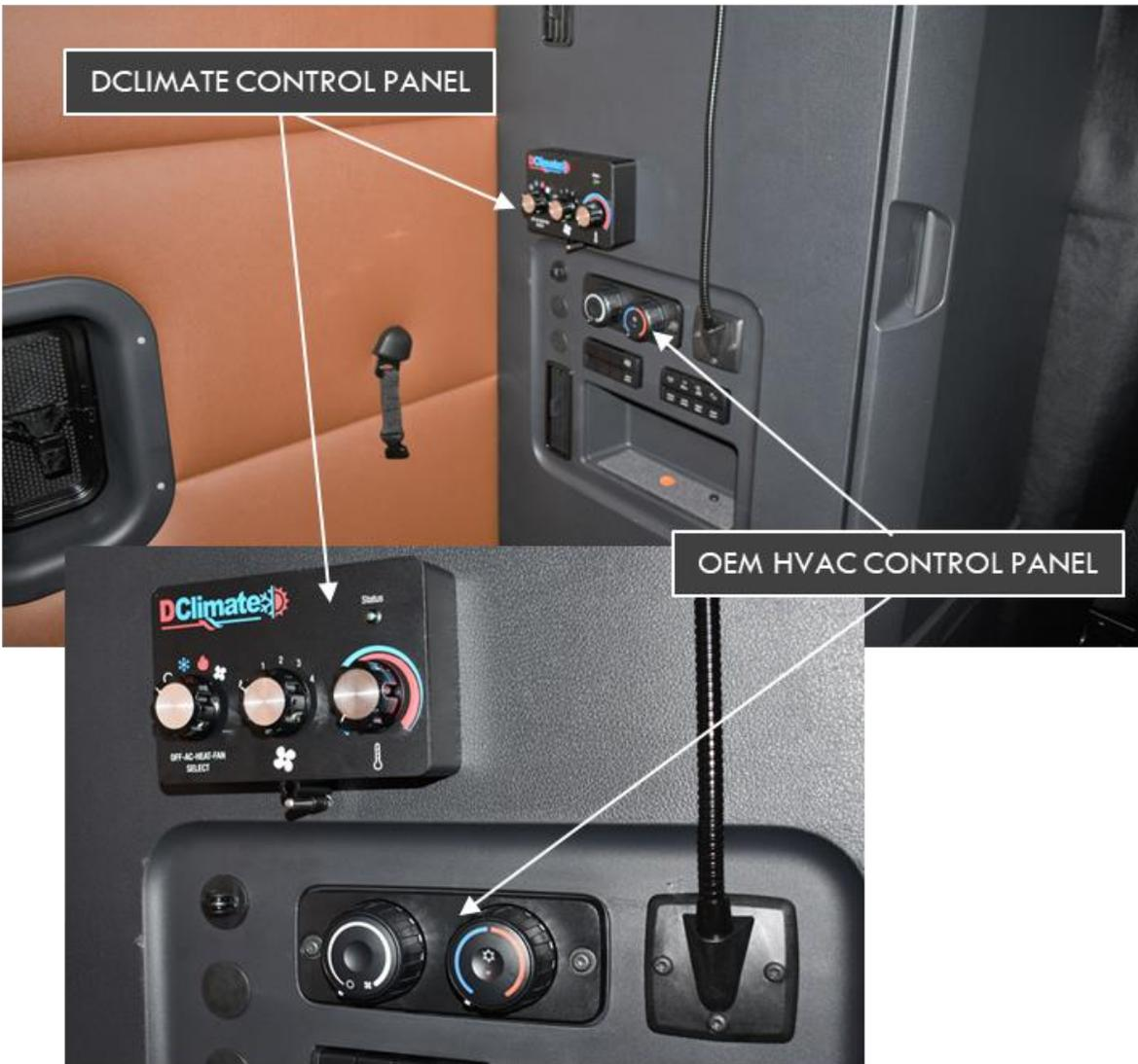
The DClimate system will only operate when the Parking Brake is engaged and will automatically deactivate when the parking brake is released. When driving, the OEM bunk HVAC system should be used to heat or cool the bunk area, using the control panel shown above.
